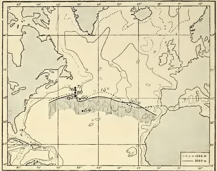
Fig. 37. Isotherm 15° and isohaline 36 ‰ 100 metres below surface. Stations 64—71 marked off.
