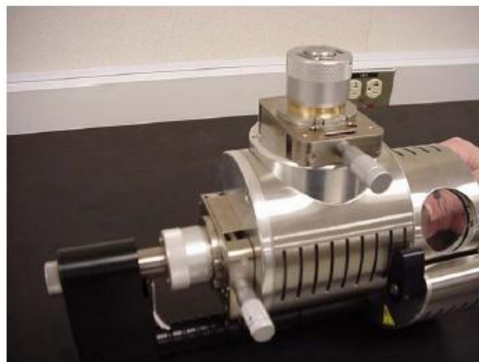
Outside of Source with articulations for the Heated Nebulizer on back and the corona needle on top
